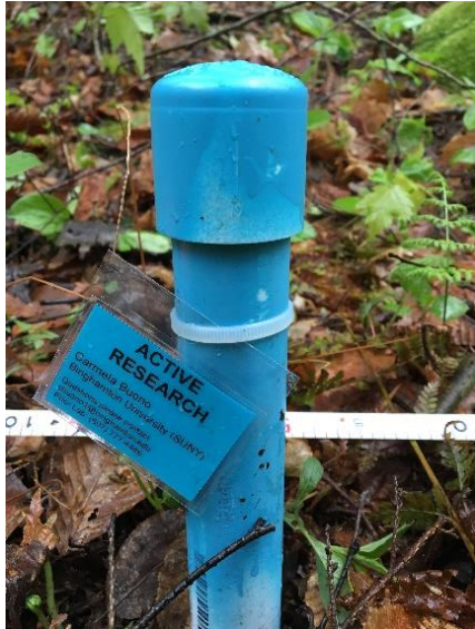
Figure 4. An image of the .5-foot-tall and 1-inch wide PVC posts that will be used to identify the ends of the study transects. In addition, these PVC posts are blue and have contact and identification information attached to them.
